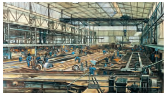
In this drawing from 1916, workers are building turntables that were used to rotate locomotives and other rail vehicles.
