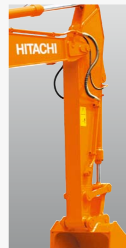
Attachment basic piping
