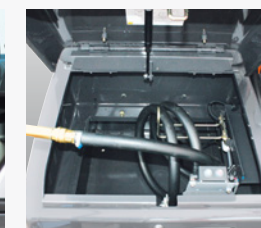
Electric fuel refilling pump
