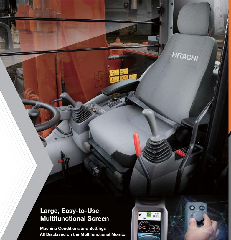
The new multi-language, multifunction monitoring system comprises a 7-inch high-resolution color monitor and a multifunctional controller. The monitor allows the operator to check varying operating variables: hydraulic oil temperature, fuel level, work mode, full-auto air conditioner, AM/FM radio, rear view.
