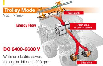
directing power only to the auxiliaries and the hydraulic pump - even when the machine is being driven uphill under load.
