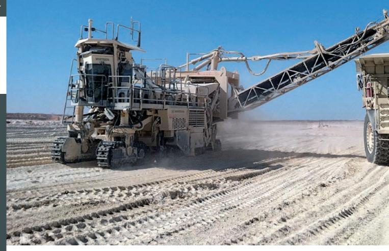
1 | The highcapacity discharge conveyor can be slewed about 90° to the left...
