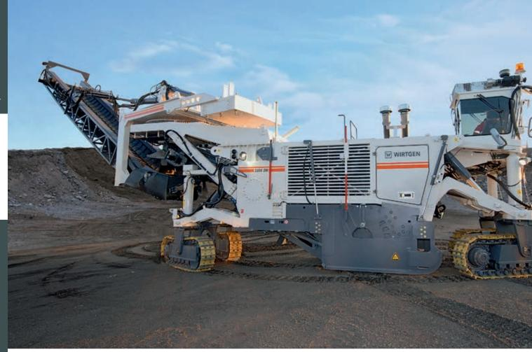
Three different steering modes optimize manoeuvrability in restricted space conditions.
