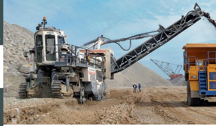
1 | Selective mining enables the 2500 SM to mine oil shale in separate layers.
