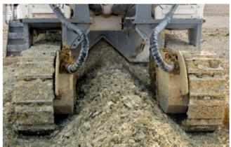
3 | When operated in windrowing mode, the adjustable scraper blade enables the track units to travel on even ground.
